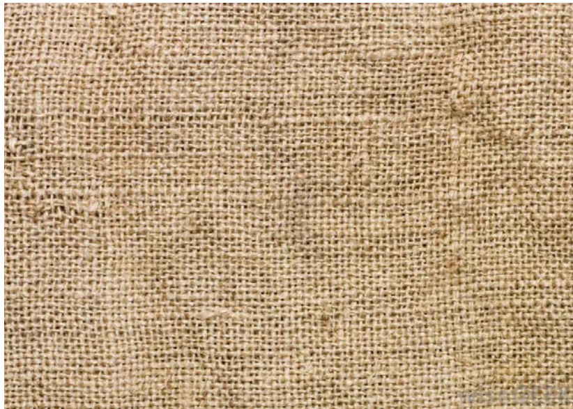
Figure 2.5 Burlap created from jute
