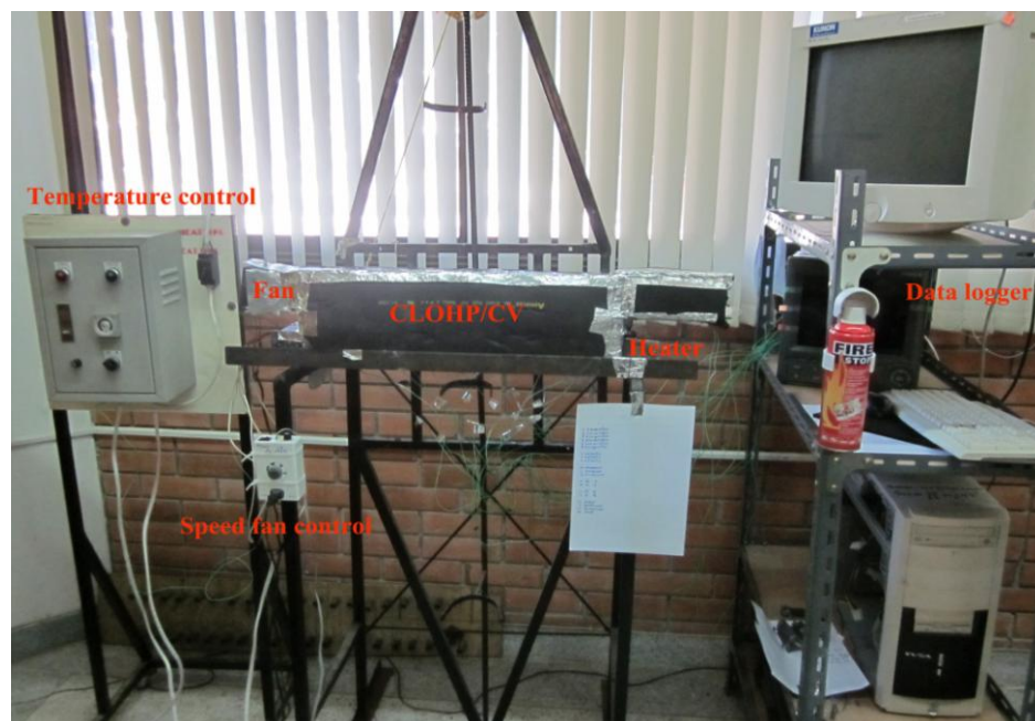
Figure 3.14 Experimental setup for internal pressure testing
