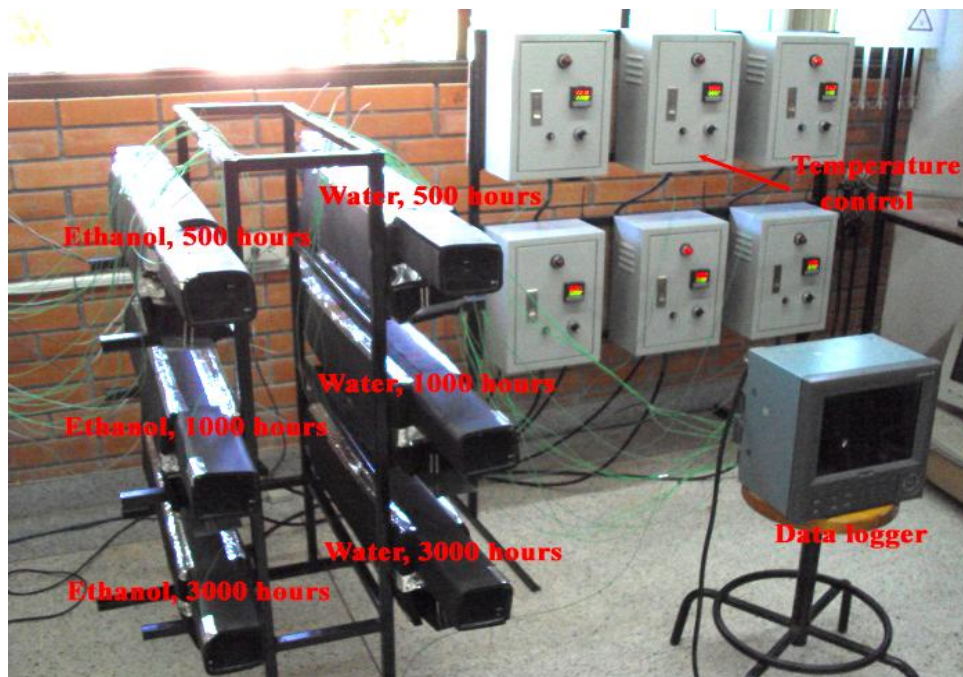
Figure 3.16 Experimental setup for internal corrosion testing
