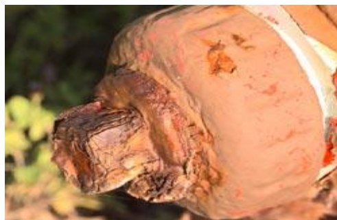
Figure 2.9 Exfoliation corrosion ( http://corrosion.ksc.nasa.gov/intercor.htm ) [48b]
