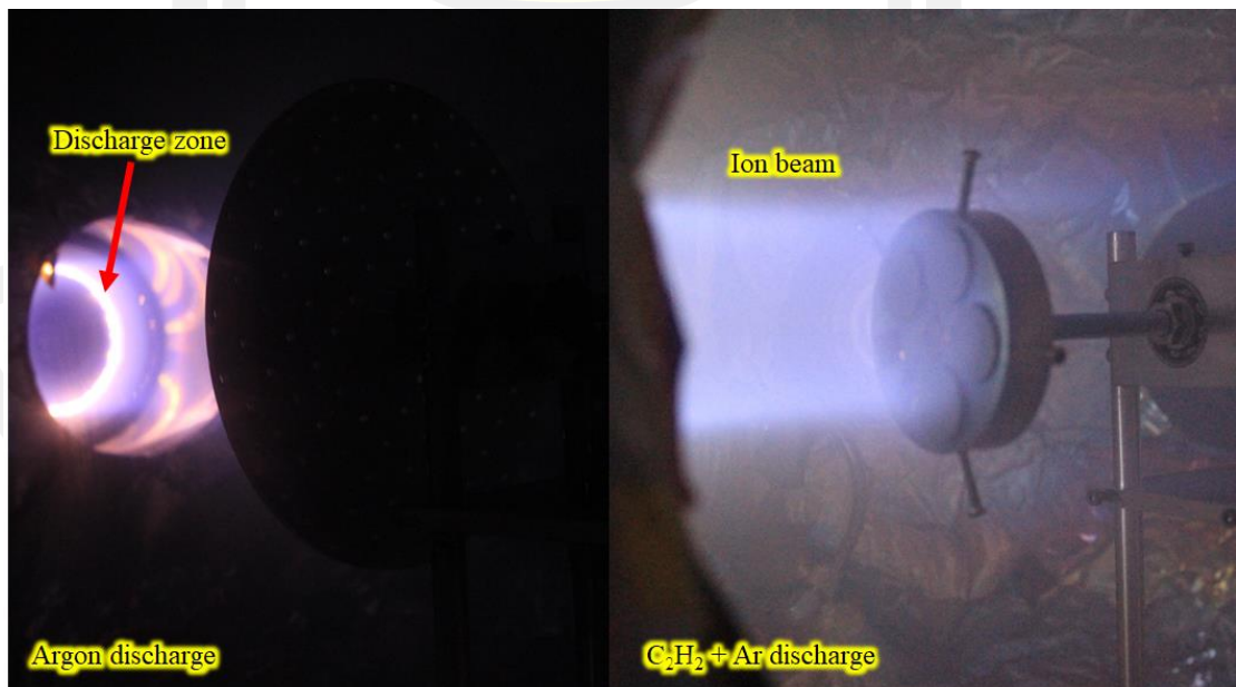
Figure 3.13 The plasma characteristic generated using an ALIS.
