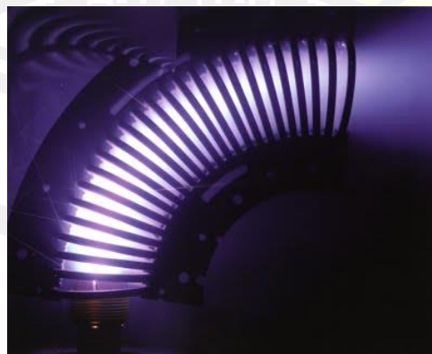
Figure 2.13 Freestanding 90° filter, operating with the arc current (200 A), Platinum plasma. [112].
