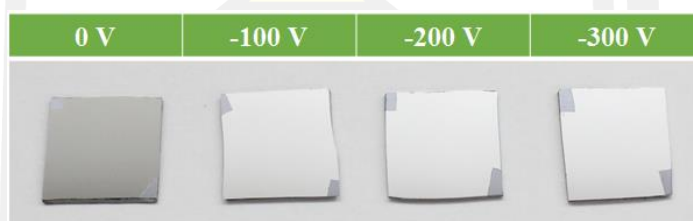
Figure 4.73 The Cr films deposited on Si substrate using HiPIMS deposition by varying substrate bias potential.
