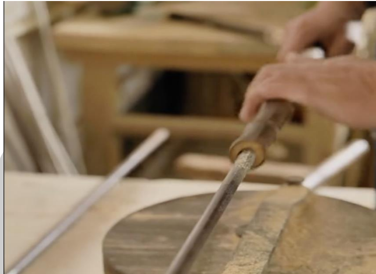
Figure 21. Sanding the inner wall
