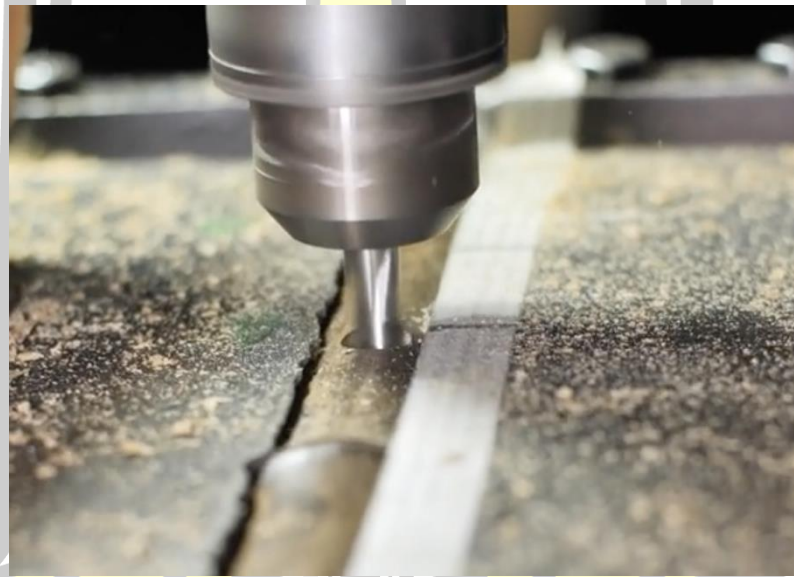
Figure 24. Drilling the holes
