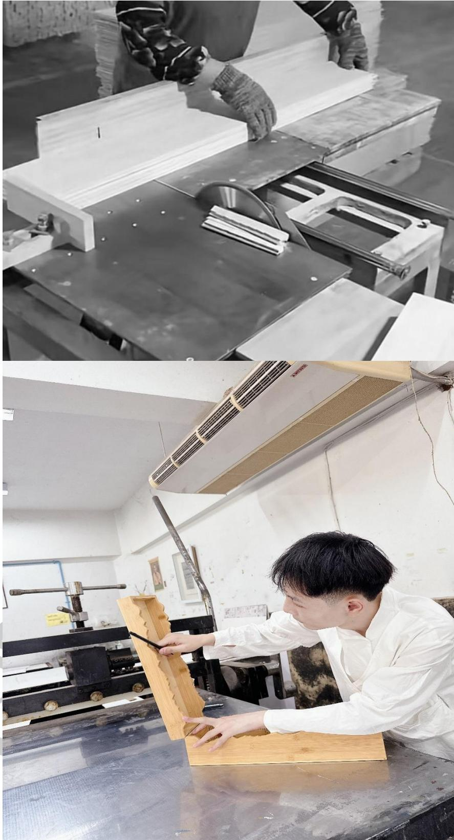
*Figure 109 Cutting of rice husk boards*
