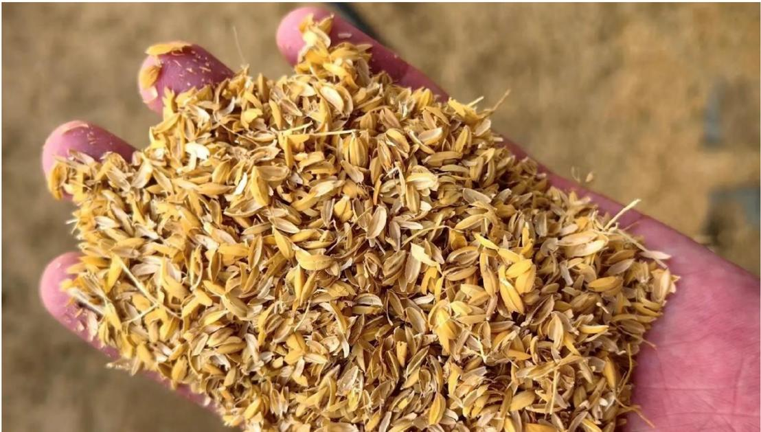
*Figure 40* Rice husk before mechanical milling
