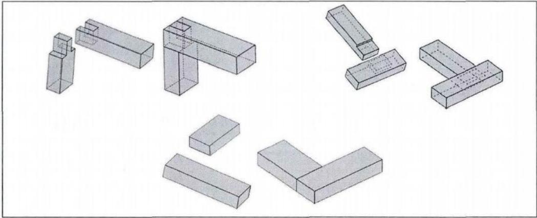
Figure 103 Selected mortise and tenon joints
