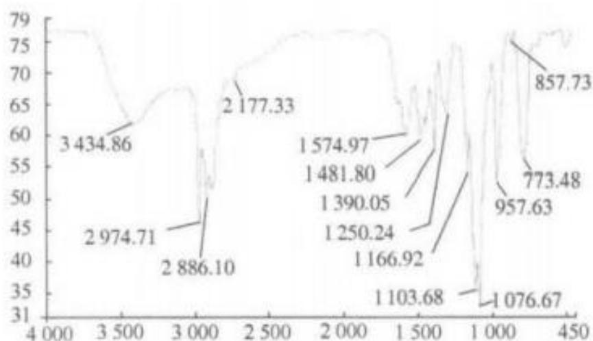
*Figure 55 Infrared Spectra of Silane Coupling Agents*
