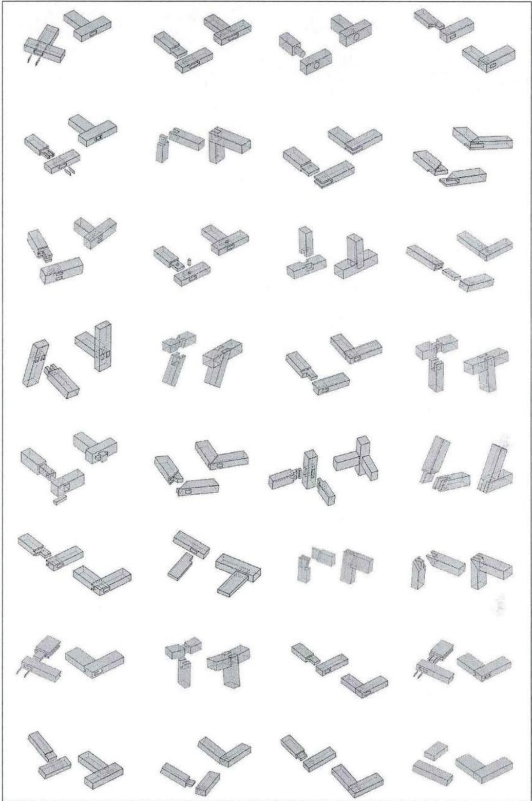
Figure 102 Structure of mortise and tenon joint
