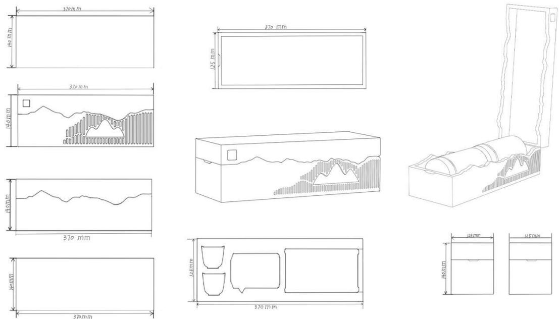
*Figure 104 Sketch of the box body design of the packaging box*
