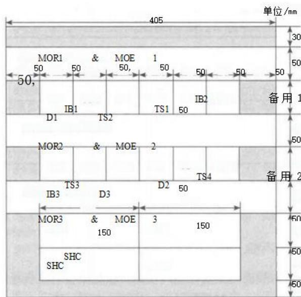
Figure 62 Specimen Preparation
